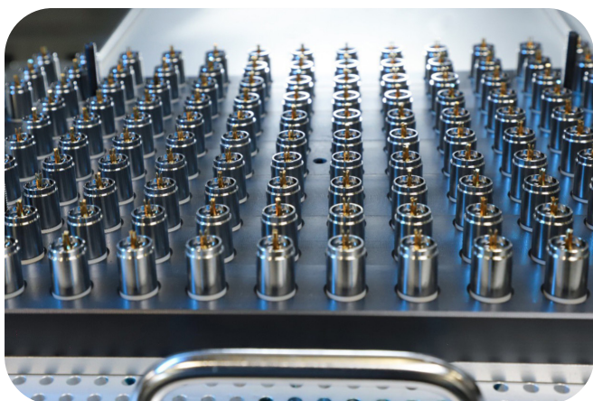
Subcontracted potting of medical sensors from ifm electronic (Tett nang) at Dipotec.
