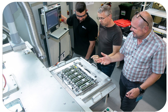
Supporting product ramp-up through subcontracted potting: Leo Gindele and Lothar Gschwind from ifm ecomatic review vacuum-potted I/O modules for mobile machinery together with Alessandro Vogl from Dipotec.
