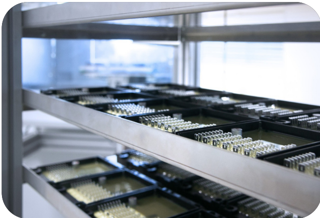
Vacuum potting of various control unit variants in an Atlas Copco vacuum potting system at ifm's Kressbronn facility.
